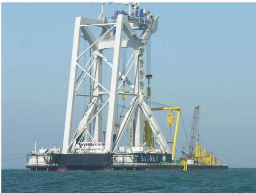
Figure 2. The heavy lift vessel *Svanen* during piling.
